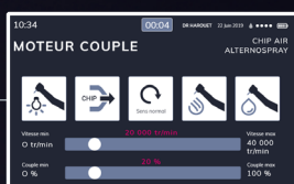
MX INDUCTION MOTOR Micromotor speed display and preselection. Torque adjustment, and auto-reverse and auto-forward functions.
